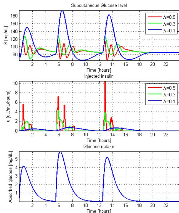
Figure 2. BG level ( $G(t)$ ) with PID-type control, at heavy glucose load [Control parameters:  $\Lambda = 0.08$ ,  $A_{ctrl} = \frac{1}{10|K_{ctrl}|} = 5 \cdot 10^{-4}$ ,  $K_{ctrl} = -200$ ,  $B_{ctrl} = 1$ , Set-point ( $G_N$ )=100 mg/dL]
