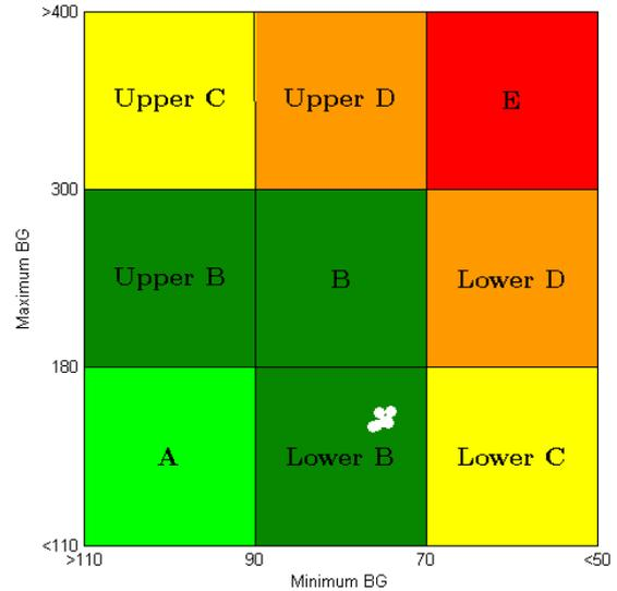
Figure 4. CVGA plot of the 8 days long simulation with the randomized feeding protocol. [Control parameters:  $\Lambda = 0.1$ ,  $A_{ctrl} = \frac{1}{10|K_{ctrl}|} = 5 \cdot 10^{-4}$ ,  $K_{ctrl} = -200$ ,  $B_{ctrl} = 1$ , Set-point ( $G_N$ )=100 mg/dL ]
