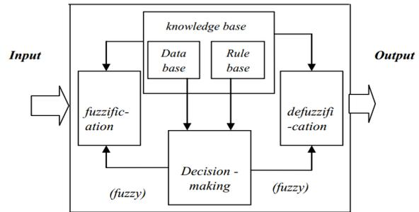
Figure 2. Schematic figure of a general fuzzy controller [15]
