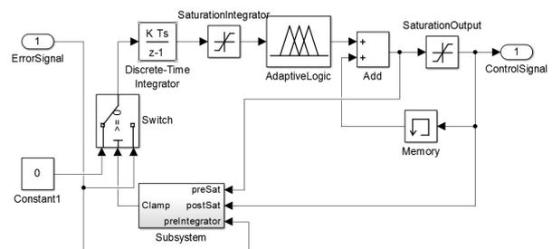
Figure 4. The developed adaptive fuzzy control scheme
