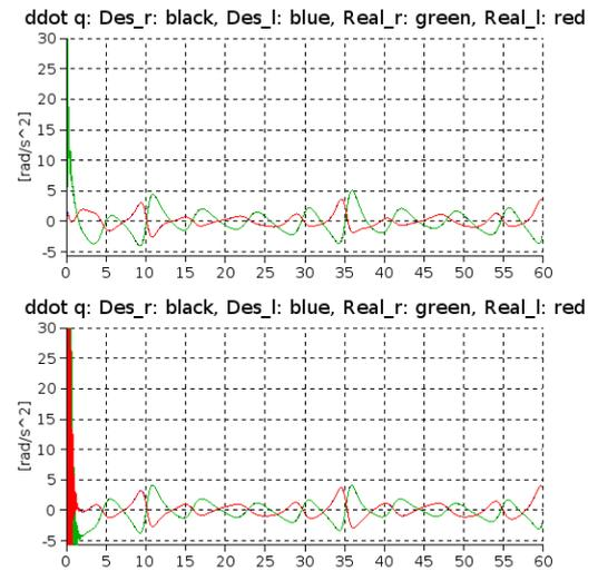
Fig. 6. The “Desired” and the *simulated* “Real” second time-derivatives of the wheels’ axes versus time in [s] units for  $\Lambda = 0.5 \text{ s}^{-1}$  (upper chart) and  $\Lambda = 1 \text{ s}^{-1}$  (lower chart). [ $\ddot{q}_r^{Des}$ : black line,  $\ddot{q}_r^{Real}$ : green line,  $\ddot{q}_l^{Des}$ : blue line,  $\ddot{q}_l^{Real}$ : red line.]
