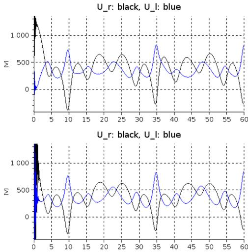
Fig. 4. The control voltages versus time in [s] for  $\Lambda = 0.5 \text{ s}^{-1}$  (upper chart) and  $\Lambda = 1 \text{ s}^{-1}$  (lower chart). [ $U_r$ : black line,  $U_l$ : blue line.]
