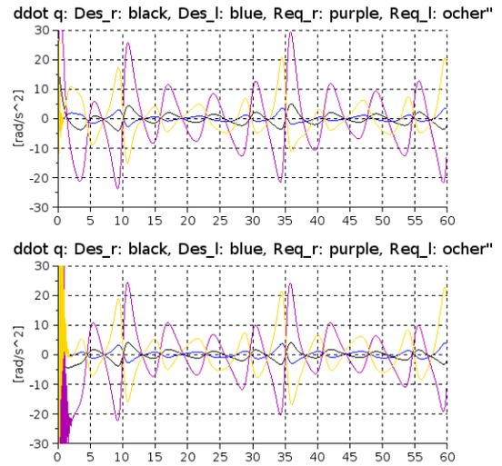
Fig. 5. The “Desired” and the *adaptively deformed* “Required” second time-derivatives of the wheels’ axes versus time in [s] units for  $\Lambda = 0.5 \text{ s}^{-1}$  (upper chart) and  $\Lambda = 1 \text{ s}^{-1}$  (lower chart). [ $\ddot{q}_r^{Des}$ : black line,  $\ddot{q}_r^{Req}$ : purple line,  $\ddot{q}_l^{Des}$ : blue line,  $\ddot{q}_l^{Req}$ : ochre line.]
