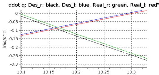
Fig. 7. The “Desired” and the simulated “Real” second time-derivatives of the wheels’ axes versus time in [s] for  $\Lambda = 1 \text{ s}^{-1}$  [ $\ddot{q}_r^{Des}$ : black line,  $\ddot{q}_r^{Real}$ : green line,  $\ddot{q}_l^{Des}$ : blue line,  $\ddot{q}_l^{Real}$ : red line, zoomed excerpts.]
