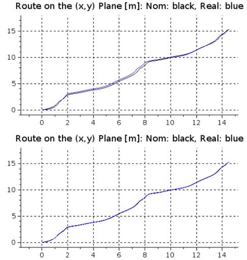
Fig. 1. Tracking of the trajectory in the  $(x, y)$  plane for  $\Lambda = 0.5 s^{-1}$  (upper chart) and  $\Lambda = 1 s^{-1}$  (lower chart). [The nominal trajectory: black line, the simulated one: blue line.]
