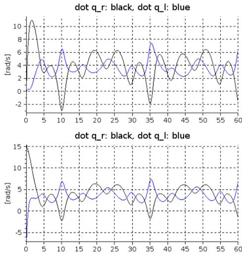
Fig. 3. The rotary speed of the wheels for  $\Lambda = 0.5 \text{ s}^{-1}$  (upper chart) and  $\Lambda = 1 \text{ s}^{-1}$  (lower chart). [ $\dot{q}_r$ : black line,  $\dot{q}_l$ : blue line, time in [s] in the horizontal axes.]
